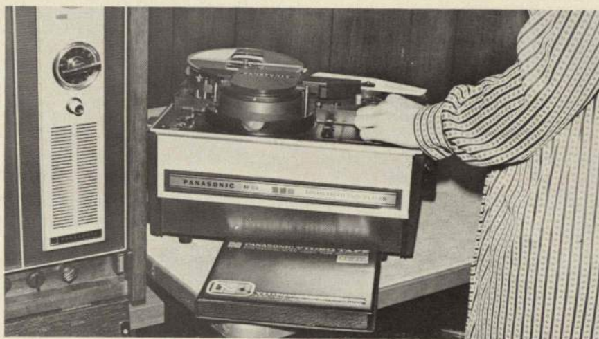
Above: The threading and operation of the video-tape machine can be handled easily by anyone conversant with the standard reel-to-reel audio tape recorder.
